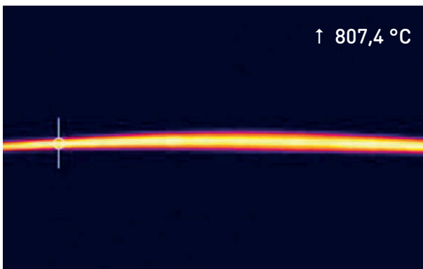
thermographic measurement on a loaded wire
